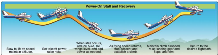
FAA Airplane Flying Handbook Figure 4-8 Power on stall
