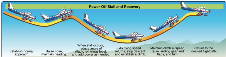
FAA Airplane Flying Handbook Figure 4-7 Power Off Stall
